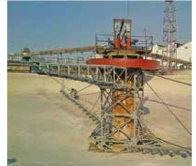
▲ A refurbished 45.7 m diameter thickener
