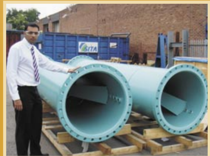
Process engineer Irfan Rehman with static mixer.
