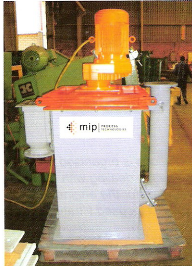
A 300 litre test attrition scrubber designed and built by MIP for trials in its pilot plant.
