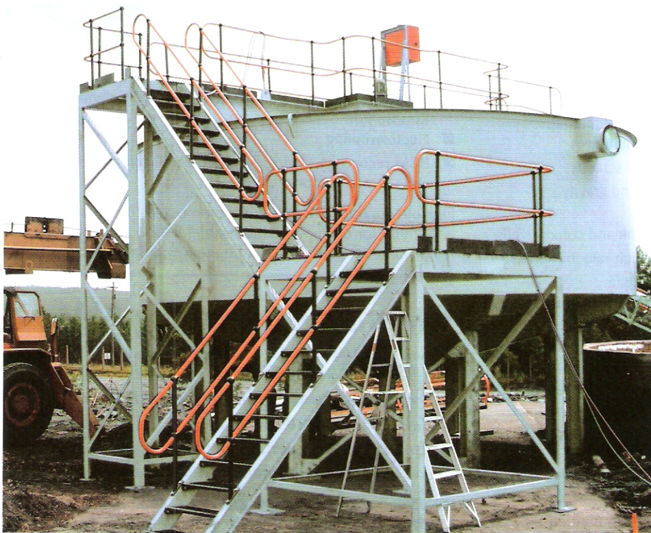
An 8 m thickener designed, built and installed by MIP in the Witbank area.
