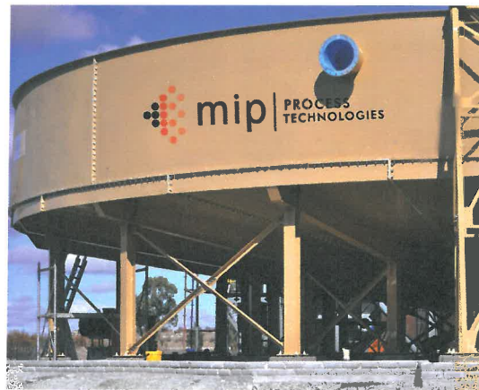
21 m diameter MIP gold thickener from bolted construction.
